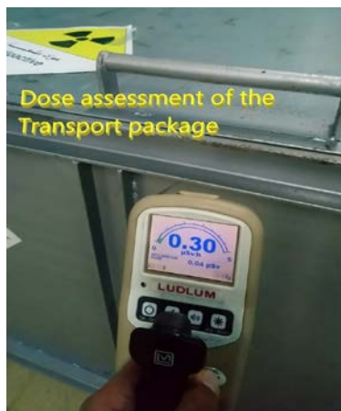
Figure 2: Dose assessment of the transport package
