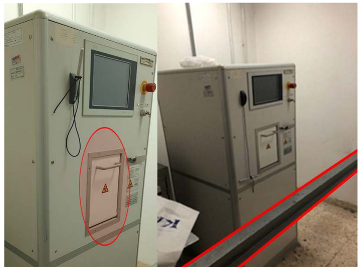
Figure 1: Old blood irradiator with a Cs-137 source (activity – 1200 Ci)
